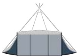
Wall panels and Infill panels used under a raised brim. Adds 28% more usable floor area.
